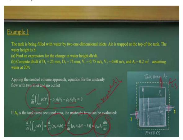
If it is that, apply the Reynolds transport theorems, okay? You apply the Reynolds transport theorems. You have the inflow and the outflow. There is no outflow in this case. In both the
