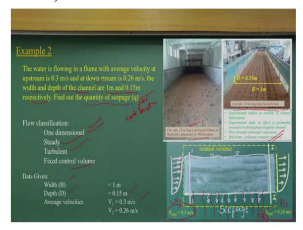
The water is flowing in a flume with a downward seepage average velocity at upstream is 0.3 m/s and at down stream is 0.26 m/s. the width and depth of the channel are 1m and 0.15m respectively. Find out the quantity of seepage (q).
