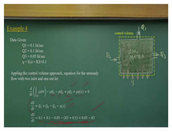
Now, if I substitute this equation, if you look at these inflows are the negative, outflows are positive, and Qx is the function of this. So, Appling the control volume approach, equation for the unsteady flow with two inlet and one out let
