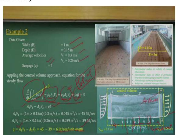
Now, we are getting this width and depth. We have the velocity, then we are looking at the seepage rate. You can see I apply the mass conservation equations. Data Given:
