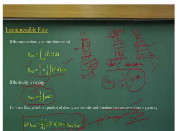
So, that way, whenever you take fluid mechanics problems, first you think what could be approximate velocity field, what could be the velocity direction. If I assume the flow is one dimensional, is it enough for me that one dimensional flow is okay for us or not, for that problem or not, or you need to have two-dimensional velocity fields, or what could be the direction, whether it is a direction with respect to the control surface normal vectors.
